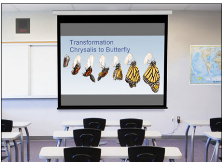
When projecting images from a source with a wide aspect ratio onto a 4:3 screen, the projector reduces the image to use only 75% of the screen area. Also, wide-screen projection makes it possible to display larger images where the room for the screen height is limited.
