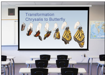
When projecting images from a source with a wide aspect ratio onto a 4:3 screen, the projector reduces the image to use only 75% of the screen area. Also, wide-screen projection makes it possible to display larger images where the room for the screen height is limited.
